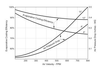
**EVAPORATIVE COOLER EFFICIENCY/A.P.D. CHART**
